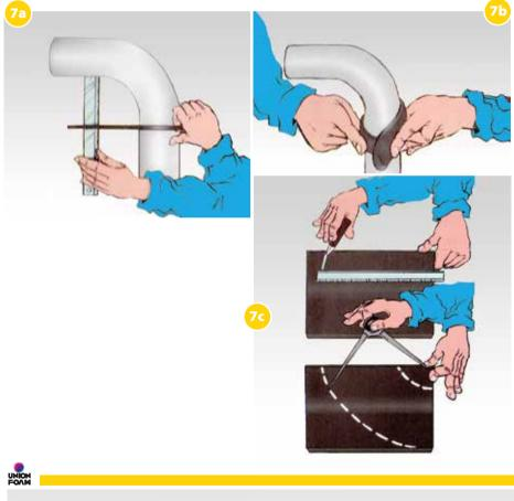
**D**) Cut the first section and then use that as a template for the second and then glue correctly and proceed as in **figs 8a, 8b, 8c, 8d, 8e**.
