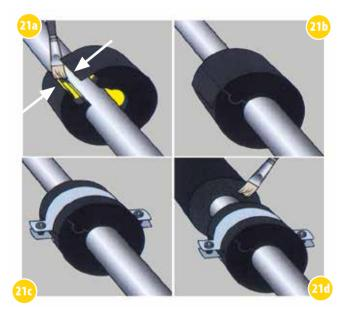
The inner core of the support, made of rigid polyurethane foam with excellent resistance to compression ensures an adequate protection to the pressure exerted by the bracket while keeping intact the sisitema insulating and optimizing the perfect functioning of the whole system.
