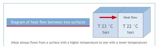
Thermal conductivity is measured in  $W/m \cdot K$  and only materials with a thermal conductivity value ( $\lambda$ ) lower than 0,100  $W/m \cdot K$  are considered as having insulating properties.
